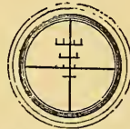
Fig. 72.—Rock Crystal Disk cross-hairs, showing elevation and wind-gauge.
